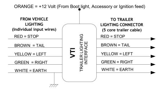
The VTI powers the trailer lighting circuits without loading the vehicle lighting circuits. It requires a separate power feed from the boot light feed or an ignition / auxiliary feed.
